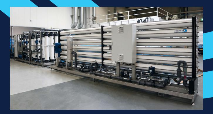
mains water to produce irrigation water.' Our concept can easily be configured for this on a modular basis, depending on the size of the horticultural business. This also makes it possible to supply clean water to multiple greenhouses with just one system.
