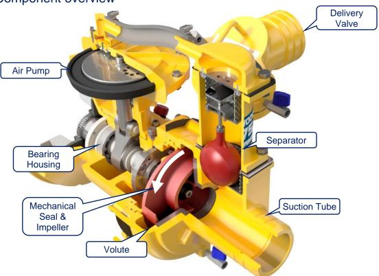
Figure 1: Body unit components. Direction of Rotation (DoR) indicated by white arrow.
