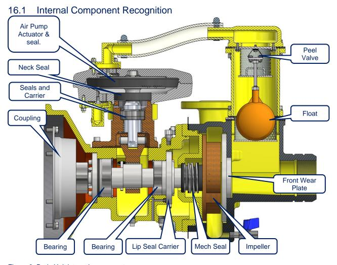
Figure 9: Body Unit internal components.
