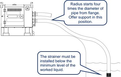
Figure 5: Correct suction line installation.
