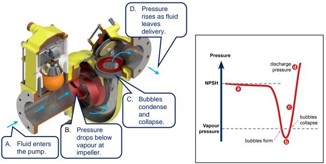
Figure 7: In this situation, the pressure at the impeller has dropped below that of the liquid, causing bubbles and subsequently cavitation to occur. This is not an ideal circumstance.
