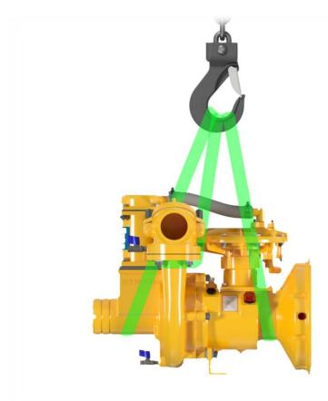
Figure 3: Strop positions when lifting the body unit.
