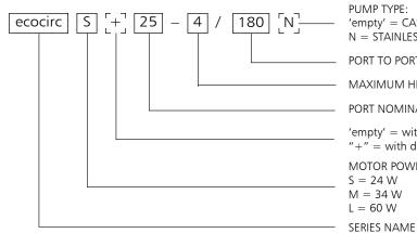
PUMP TYPE: 'empty' = CAST IRON N = STAINLESS STEEL (for Domestic Hot Water) PORT TO PORT DISTANCE IN mm.
