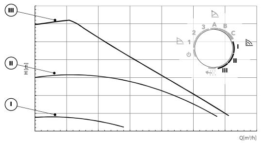
Constant speed control is the most common when used in the primary or boiler loop in a primary/secondary hydronic system.
