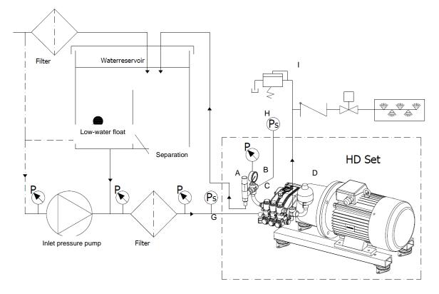
Figure 3 HD pump set flow diagram
